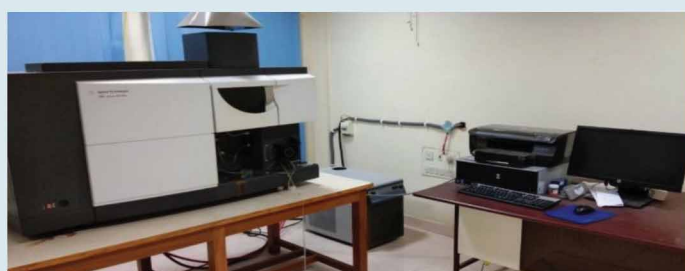
Inductively Coupled Plasma Optical-Emission spectroscopy (ICP-OES) Make: Agilent USA, Model: 700 Series ICP-OES
