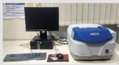
DR - UV - VIS SPECTROPHOTOMETER (established by Physics Department and sponsored by SERB)
