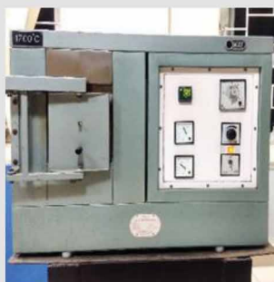
MUFFLE FURNACE (1500°C)
