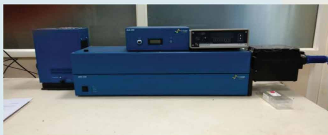
Circular Dichroism-Optical Rotatory Dispersion (CD-ORD) Spectrometer Make: Bio Logic Czech, Model: MOS-500
