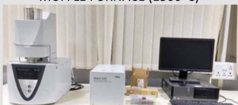
THERMO-GRAVIMETRIC & DIFFERENTIAL THERMAL ANALYZER (Model: STA 2500 Regulus, Make: NETZSCH) Max Temperature – 1600°C
