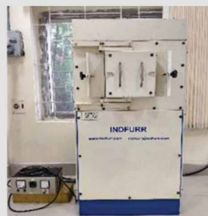
MUFFLE FURNACE (1700°C)
