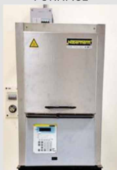
MUFFLE FURNACE (1800°C)
