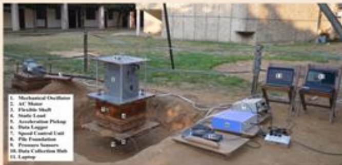
PILE VIBRATION TESTING SETUP
