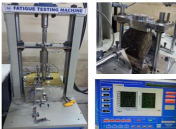
Transportation Engineering Laboratory- Fatigue Testing Machine Test Setup (Plan Grants)
