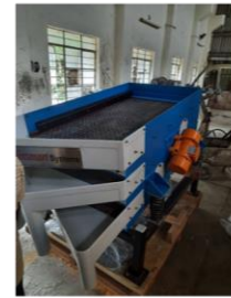
Concrete Laboratory-Segregator (SRIC)
