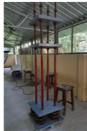
Concrete Laboratory-Creep Testing Equipment (Plan Grants)
