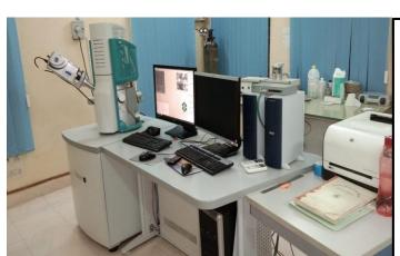
**Scanning Electron Microscope (SEM)**
