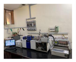
Equipment Name: DUEL-INLET ISOTOPE RATIO MASS SPECTROMETER Make: GB instruments Model: Isoprime JB-202 Application: It is used for analyzing stable isotopes in
