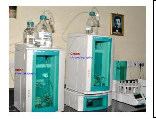
Equipment Name: ION-CHROMATOGRAPHY <u>Make:</u> Metrohm <u>Model:</u> 882 Compact IC Plus <u>Application:</u> It is used for the determination of anion and few cations in water samples. It is useful in the environmental sciences.
