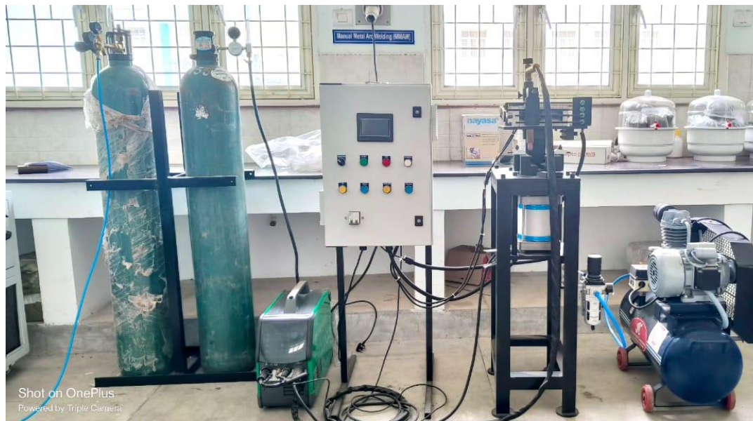
Varestraint testing equipment
