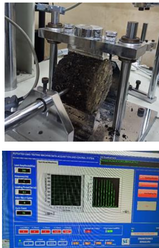
Transportation Engineering Laboratory- Fatigue Testing Machine Test Setup (Plan Grants)
