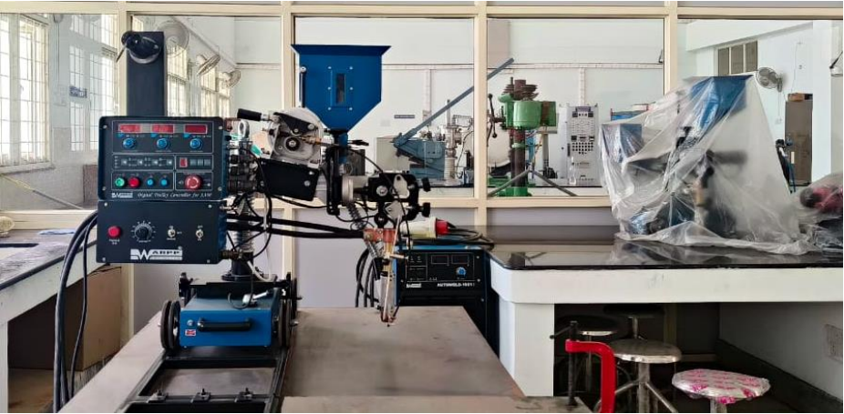
Sub merged arc welding (SAW)
