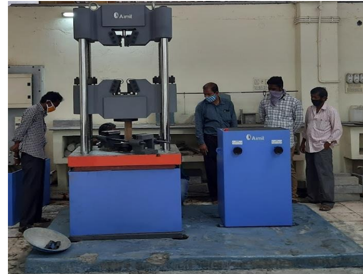
Structures Laboratory- 100 Ton UTM (TEQIP-III)
