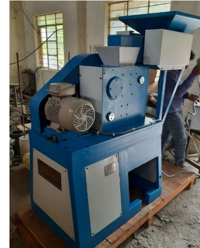
Concrete Laboratory- Jaw Crusher (SRIC)
