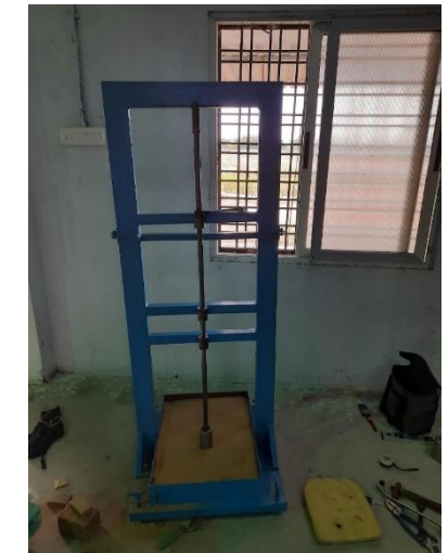
Structures & Dynamics Laboratory- Drop Weight Impact Tester (IMPRINT-2)
