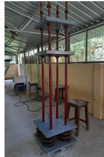
Concrete Laboratory-Creep Testing Equipment (Plan Grants)
