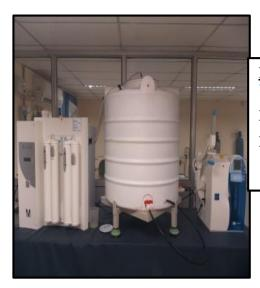
Equipment Name: Ultrapure Water System Milli Q Direct 8 Elix Make: Millipore Pvt. Ltd Model: Milli Q Direct 8 ELIX
