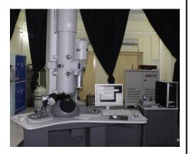
**Equipment Name: High Resolution Transmission Electron Microscopy (HR-TEM)**
